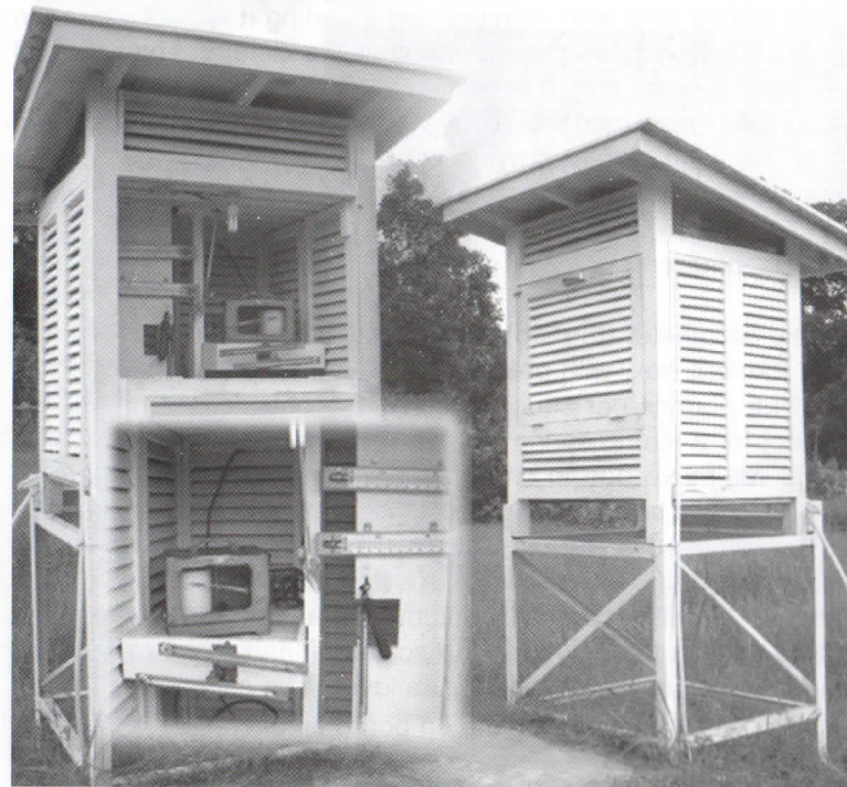
Fig. 3. Thermometer Shelter or Screen. In the Northern Hemisphere its door faces north to prevent the sun's rays from directly affecting the instrument readings whenever it is opened
