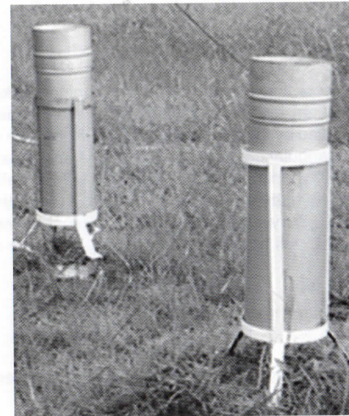
Fig. 8. An 8-inch rain gauge and its parts. a.) measuring stick; b.) tube; c.) receiver and d.) overflow can.
