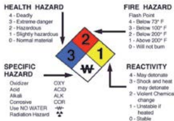
Figure 5.2 Hazardous material identification symbol showing the types of active hazard that could be created by an accidental release
