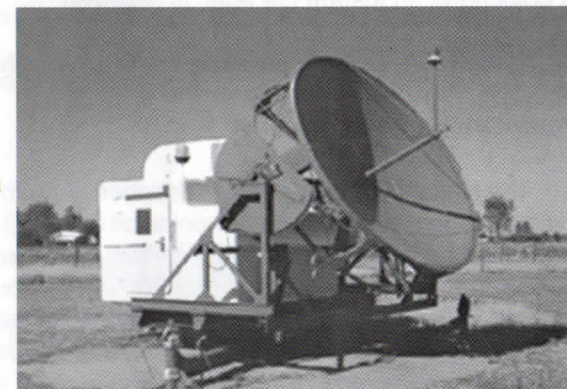
Fig. 13. Wind Finding Radar Antenna
