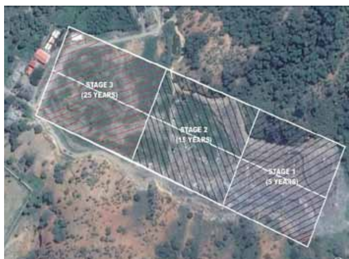
Cell staging over the landfill life.
