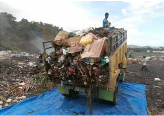
Dumping a full load to measure mass once volume has been determined in situ, after which waste density is checked.
