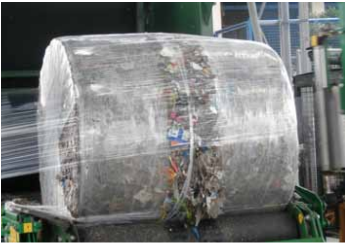
Wrapping a bale of refuse-derived fuel.
